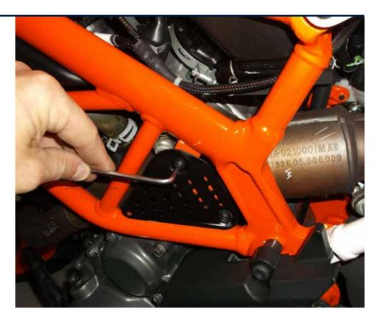
Use allen key (hex key) #5 to remove the clamp bolts
