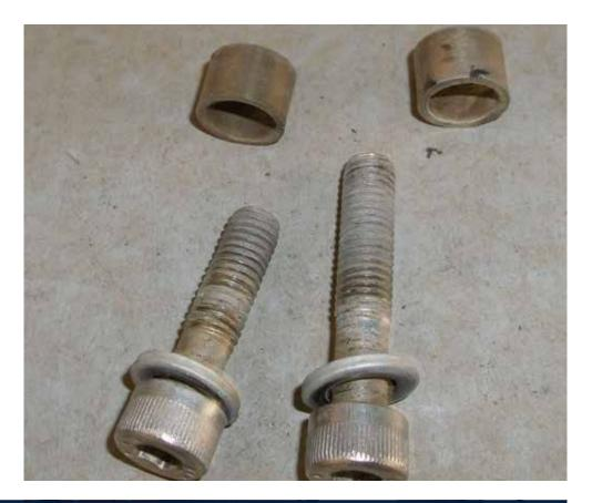
Use 8mm and 12mm key to remove the mid muffler screws
